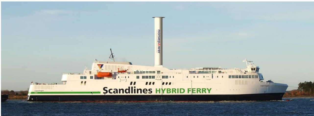
An illustration of M/V Copenhagen with a Norsepower Rotor Sail
